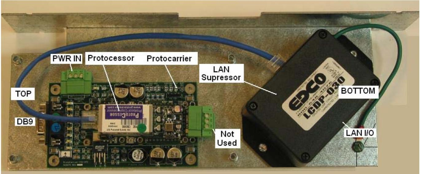
Figure 2: BACPac Ethernet Module
