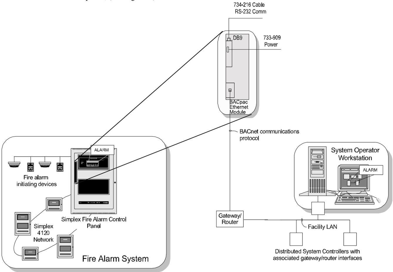
Figure 1: BACPac Ethernet Module Location Within the Control Panel
