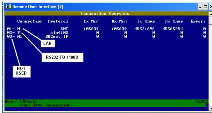
Figure 12: BACpac Interface Communications Data (Selection “O”)
