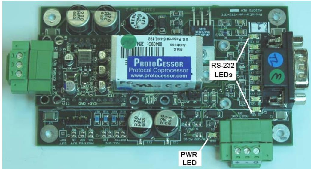
Figure 3: Protoccarrier Status LEDs
