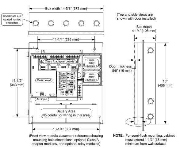
**NOTE:** A system ground must be provided for Earth Detection and transient protection devices. This connection shall be made to an approved, dedicated Earth connection per NFPA 70, Article 250, and NFPA 780.
