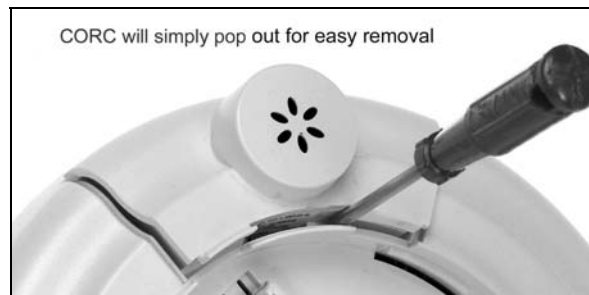
Figure 3-9. Removing the CORC from the Sensor Base
